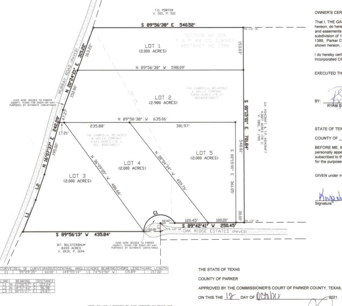
BEARING BASIS: TEXAS STATE PLANE COORDINATE SYSTEM, NAD83 NORTH CENTRAL TX ZONE, US SURVEY FOOT
