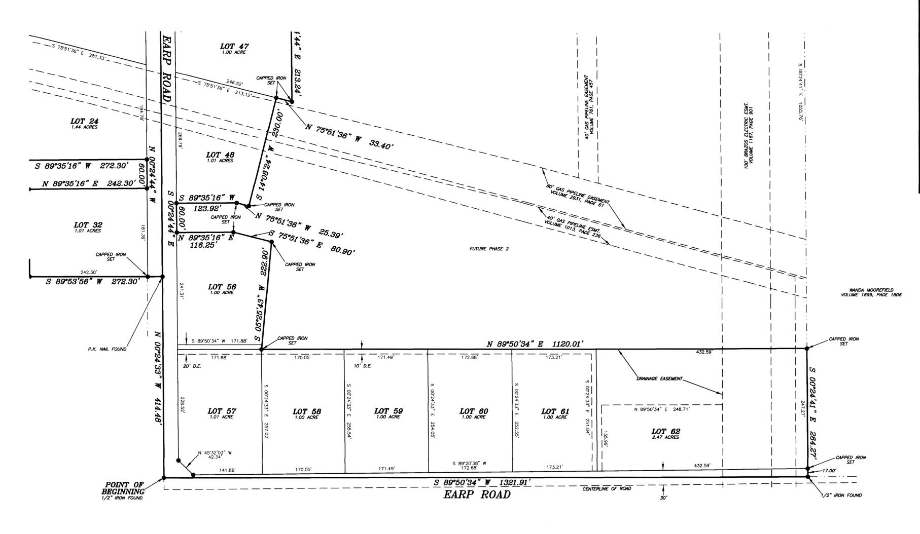
BASIS OF BEARING PER G.P.S. OBSERVATIONS. TRIMBLE RTK NETWORK. TEXAS STATE PLANE COORDINATE SYSTEM, NORTH CENTRAL ZONE 4202, N.A.D. 1983.
