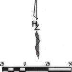
SCALE: 1" = 50' PLEASE REFER TO BAR SCALE, DRAWING MAY HAVE BEEN REDUCED OR ENLARGED. BASIS OF BEARINGS: Bearings are based on the Texas State Plane Coordinate System, North Central Zone (4202) North American Datum 1983 (2011). ■ HZF — 5/8" IRON ROD FOUND WITH PLASTIC CAP STAMPED "HUITT-ZOLLARS"
