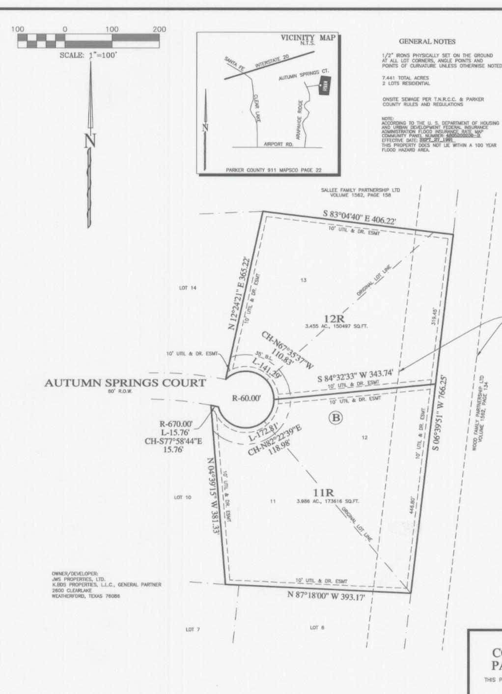
1/2" IRONS PHYSICALLY SET ON THE GROUND AT ALL LOT CORNERS, ANGLE POINTS AND POINTS OF CURVATURE UNLESS OTHERWISE NOTED
