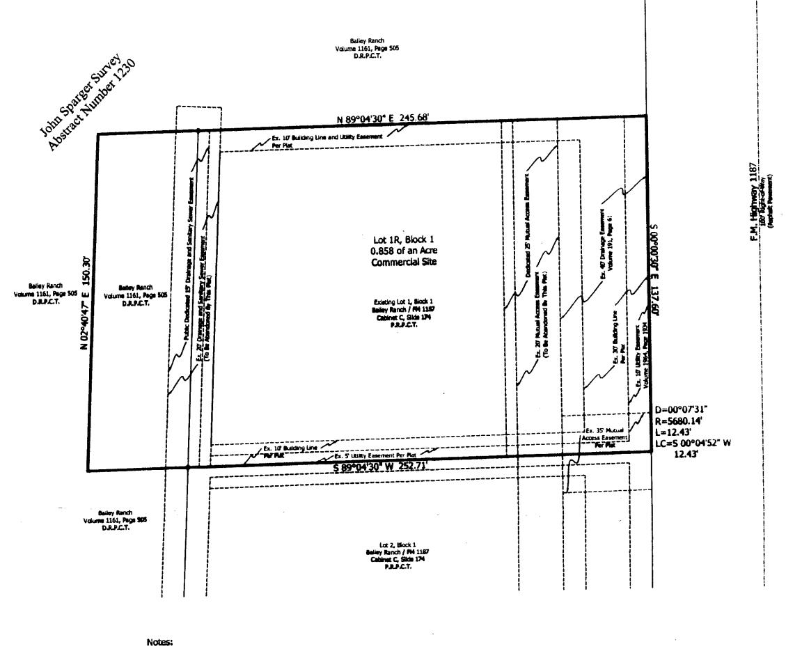
1. The basis of bearings is the Texas State Plane Coordinate System, North American Datum of 1983, North Central Zone determined by GPS observation.
