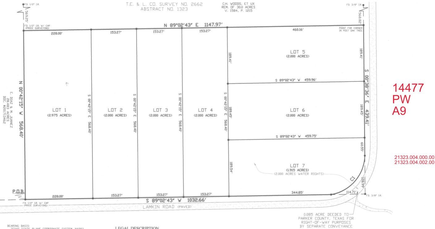
BEARING BASIS: TEXAS STATE PLANE COORDINATE SYSTEM, NAD83 NORTH CENTRAL TX ZONE, US SURVEY FOOT
