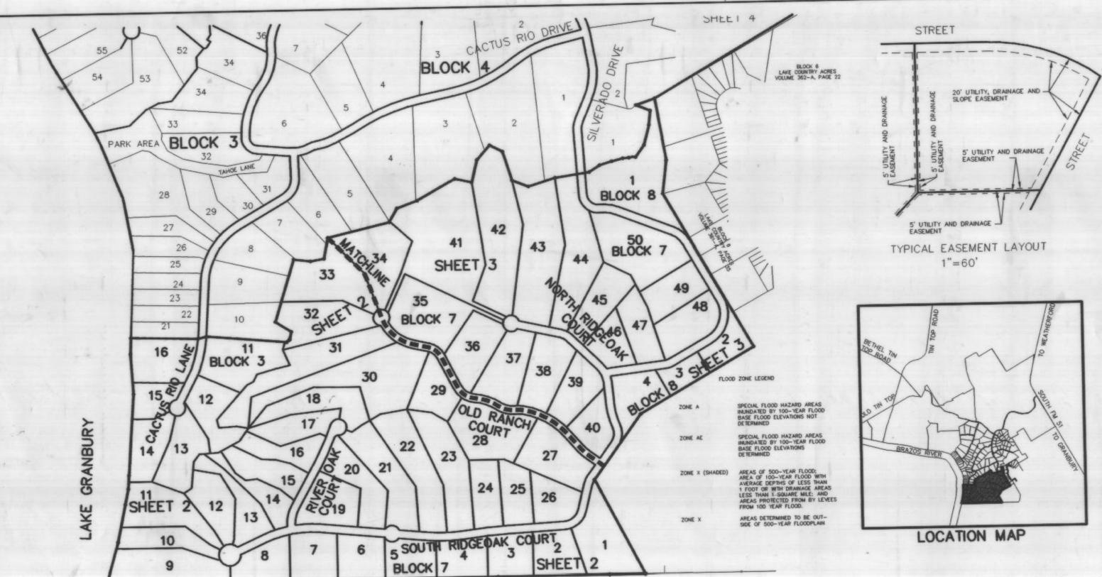
1.) A 20 FOOT UTILITY, DRAINAGE AND SLOPE EASEMENT ADJOINING ALL RIGHT OF WAYS IS HEREBY DEDICATED. A 5 FOOT SIDE LOT UTILITY AND DRAINAGE EASEMENT IS HEREBY DEDICATED. 2.) A PORTION OF THIS PLAT ARE SITUATED IN FLOOD ZONE AE (100 YR, FLOOD) PER FEMA MAP NO. 480520 0275 B, EFFECTIVE DATE SEPTEMBER 27, 1991. 3.) THE DEVELOPMENT OF INDIVIDUAL OWNERS SHALL NOT BLOCK
