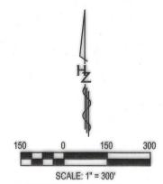
PLEASE REFER TO BAR SCALE. DRAWING MAY HAVE BEEN REDUCED OR ENLARGED BASIS OF BEARINGS: Bearings are based on the Texas State Plane Coordinate System, North Central Zone (4202) North American Datum 1983 (2011).
