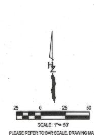
PLEASE REFER TO BAR SCALE. DRAWING MAY HAVE BEEN REDUCED OR ENLARGED. BASIS OF BEARINGS: Bearings are based on the Texas State Plane Coordinate System, North Central Zone
